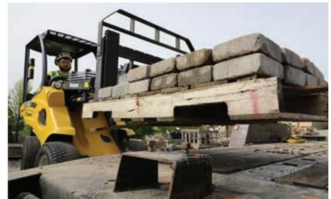
**LIFT-CAPACITY-TO-WEIGHT RATIO.** The ATX530 has a rated operating capacity (straight) of 1,343 lb (609.2 kg)\* while having a standard weight of 2760 lb (1252 kg) with rear weights and without attachments. This lift-capacity-to-weight ratio allows contractors to utilize a lighter machine while still being able to carry heavy materials on the jobsite.
