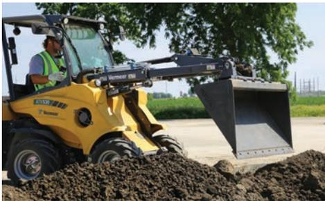
**TELESCOPIC BOOM.** The telescopic boom on the ATX530 extends 21.6 in (54.9 cm) for loading materials to a dump height of 108.3 in (275.1 cm) in hinge pin height. The telescopic boom can also aid in dumping material over the back of a retaining wall or grabbing material over an obstruction.
