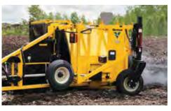
**HEAVY-DUTY FRAME.** Constructed of four members of 4" x 3" x 3/16" (10.2 cm x 7.6 cm x .5 cm) structural steel tubing and steel plate. Heavy-duty frame adds rigidity to the unit to help prolong the life of bearings and drum shafts.
