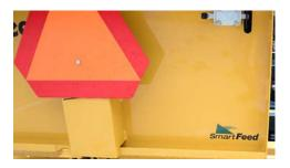
**EXCLUSIVE SMARTFEED CONTROL SYSTEM.** Helps operator productivity and reduces strain on vital engine parts, as engine rpm is monitored and feed rollers are controlled.
