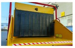
**LARGE INFEED OPENING.** 12 in x 17 in (30.5 cm x 43.2 cm) maximizes the efficiency of irregular material feeding and reduces the need to trim material before feeding it into the chipper.
