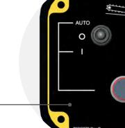
4 Hydraulic controls provide operators the ability to choose how the spout is angled and how the crop is distributed.
