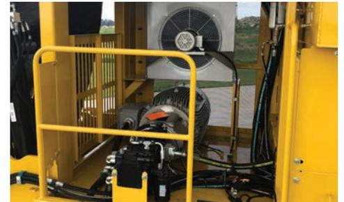
**ELECTRIC MOTORS.** Powered by two industrial-duty, fully enclosed and fan-cooled electric motors. A single 150-hp (112-kW) motor powers the hydraulic pump stack while a .75-hp (.6-kW) motor powers the cooling fan for the hydraulic system.
