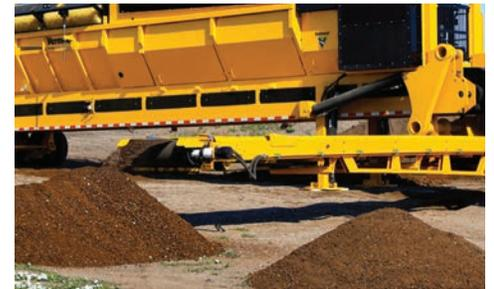
**RADIAL STACKING CONVEYOR.** The stacking conveyor with a 180-degree arc increases the amount of material being stacked on the ground. Adjustable stacking height aids with dust control and helps avoid material being blown away.
