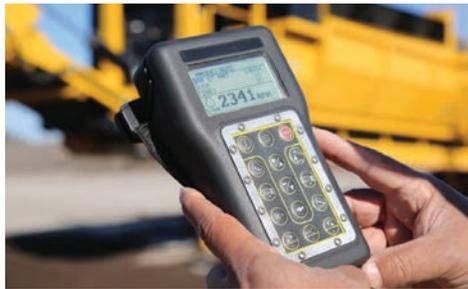
**ADVANCE CONTROLS.** Operators can control the machine through either the Vermeer DP10 display mounted on the control panel, or through a handheld transceiver remote.
