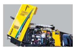
SERVICEABILITY. A one-piece, hinged hood offers durability as well as easy access to key service points.
