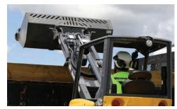
**TELESCOPIC BOOM.** The telescopic boom on the ATX850 extends 29.1 in (73.9 cm) for loading materials to a dump height of 117.3 in (297.9 cm) in hinge pin height. The telescopic boom can also aid in dumping material over the back side of a retaining wall or grabbing material over an obstruction.
