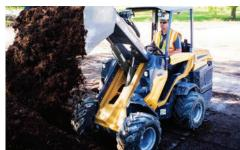
**COMPACT SIZE.** With narrow tires, the ATX850 is 42.1-in (106.9-cm) wide, while the wider tires make the machine 50.4-in (128-cm) wide. Various tire width options allow the ATX850 to fit through a standard four-foot gate for backyard access on landscape jobs. The overall length of the ATX850 is 120.3 in (305.6 cm).
