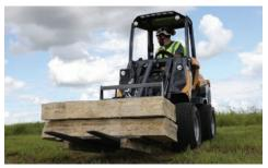
LIFT-TO-WEIGHT RATIO. The ATX850 has a rated operating capacity (straight) of 2,542 lb (1,153 kg)\* while having a standard weight of 4,145 lb (1,880 kg) with rear weights and without attachments. This lift-capacity-to-weight ratio allows contractors to utilize a lighter machine while still being able to carry heavy materials on the jobsite.
