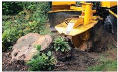
MAXIMUM CUTTING WIDTH. The SC552 reduce the operator's time repositioning the machine with a cutting height of 31 in (78.7 cm) above ground and 25 in (63.5 cm) below grade. the straight-line cutting dimension allows the operator to cut a 6 ft (1.8 m) stump without repositioning the machine.
