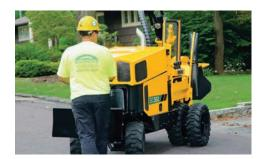
FOUR-WHEEL DRIVE WITH DIFFERENTIAL **LOCK.** With power and torques transferred to each of the four wheels, the SC552 is able to traverse in difficult terrain where the operator can engage the differential locks to maintain pulling power during uneven wheel traction path.
