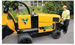
**AUXILIARY CONTROL STATION.** In narrow jobsite conditions that restrict use of the main control station, the operator can control ground drive and steering functions from this folding station mounted at the front end of the machine.
