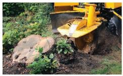
MAXIMUM CUTTING WIDTH. The SC552 reduce the operator's time repositioning the machine with a cutting height of 31 in (78.7 cm) above ground and 25 in (63.5 cm) below grade. the straight-line cutting dimension allows the operator to cut a 6 ft (1.8 m) stump without repositioning the machine.
