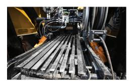
LIGHTEN YOUR LOAD. The shaker deck separates solids from liquid which helps lighten the slurry load that needs disposed of and helps extend time on the jobsite.
