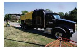
**KEEP ON RUNNING.** The hydraulic PTO helps keep you running and save time because you do not need to shift power back and forth to the vac and truck.
