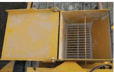
A CLEAN MIX. A wide-mouth hopper pairs with the tapered bottom rectangular tank to help prevent drilling fluid additives from settling, assist with drainage and reduce buildup.
