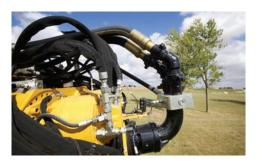
4-IN (10.2-CM) FLUID COURSE. New 4-in (10.2 cm) fluid course allows more fluid to be pumped downhole at a low pressure drop.
