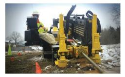
**COMPACT CONTROL.** A width of 55.5 in (141 cm) makes the D23x30DR S3 drill 24.5 in (62.2 cm) narrower than its closest competitor, offering efficient maneuverability of the machine into compact urban areas or busy neighborhoods, and convenient transportation on a trailer with other equipment.
