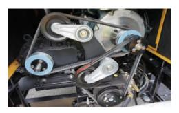
AUTO BELT TENSIONERS. Keeps proper belt tensions at all times and helps extend belt life.
