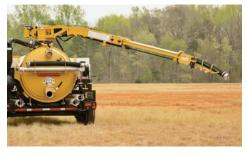
HYDRAULIC BOOM (OPTION). 4 ft or 5 ft (10.2 cm or 12.7 cm) Exclusive telescoping boom maintains hose length during extension and incorporates a remote controlled hydraulic valve for vacuum shut off. Available with manual or hydraulic rotations.
