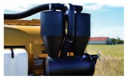
THREE-STAGE CYCLONIC FILTRATION. Engineered to help prolong filter and blower life, the system is suitable for wet and dry applications. The cyclones use a tuned vortex system in which the outer vortex spiral forces small particles to fall into a separate canister. The filtered stream then passes up through the inner cyclone tube and is carried to the final poly filter.
