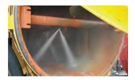
IN-TANK WASHDOWN. Delivers a high-pressure water spray to the tank interior helping simultaneously dump material and clean the inside of the tank. Minimizes cleanup time and helps remove difficult debris.
