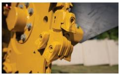
**VERMEER CUTTING SYSTEM.** The Vermeer cutting system features a patented design that solves several challenges associated with traditional cutting systems, including double-sided teeth with no pockets that need replaced, a V-profile, center core protection, minimized recirculation and ease of maintenance.
