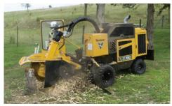
4-BAR LINKAGE. Maximize cutting width through a unique 4-bar linkage that moves the cutter wheel away from the machine as the boom drops. This helps the cutter wheel grind the stump at all maximum dimensions.
