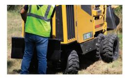
ALL-TERRAIN. With power and torque transferred to each of the four wheels, the SC1052 is able to traverse difficult and uneven ground conditions, with minimal ground disturbance. With the differential locks disengaged, maneuverability is enhanced. In difficult ground conditions, the operator can engage the differential locks to maintain pulling power during uneven wheel traction conditions.
