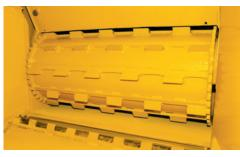
**LOWER FEED ROLLER.** The lower feed roller is offset from the upper feed roller by 10.8" (27.4 cm). Material is easily pulled to the upper feed roller, so there is less need to manually raise the upper feed roller for larger diameter material.
