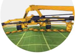
2 The hydraulic suspension system works in conjunction with the split cutter bar to reduce cutter bar weight on the ground, increase flex and allow the TM1200 to follow ground contour.
