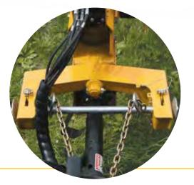
6 A patented 2-point Quick Hitch hookup is designed to allow one person to hook up the mower. It also provides high ground clearance to help avoid obstructions while in the field.
