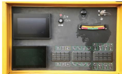
**COMPLETE CONTROL.** Optimize productivity and flexibility when operating with these two features: An industry leading, full function, wireless remote control lets you, from the cab, adjust machine settings as conditions change, including control of the infeed settings, vacuum settings, shaker table, conveyor height and more. The 7-in (18-cm) onboard color touch screen display shows machine data and allows you to intuitively set up the machine for maximum
