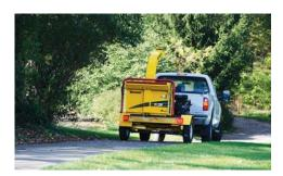
**WIDE AXLE.** Offers an ample footprint at the axle for side-to-side stability and optimizes transportability.
