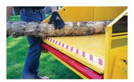
**BOTTOM FEED STOP BAR.** Strategically located to make it possible for an operator to strike the bar and shut off the feed mechanism.
