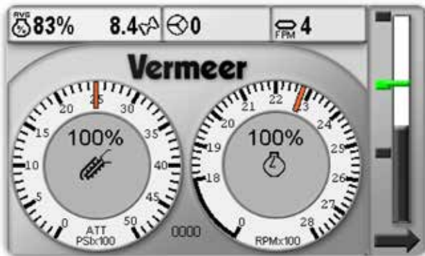
CLEANER DASH DISPLAY. Shows the operator the status of the most critical elements of machine performance.
