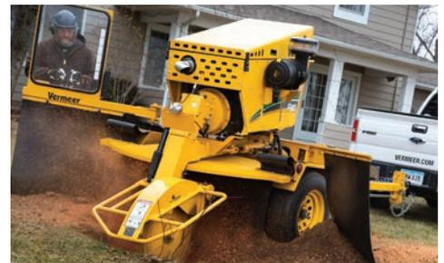
**FLOATATION TIRES.** This standard feature allows the weight of the machine to be dispersed over a larger area reducing the ground disturbance.
