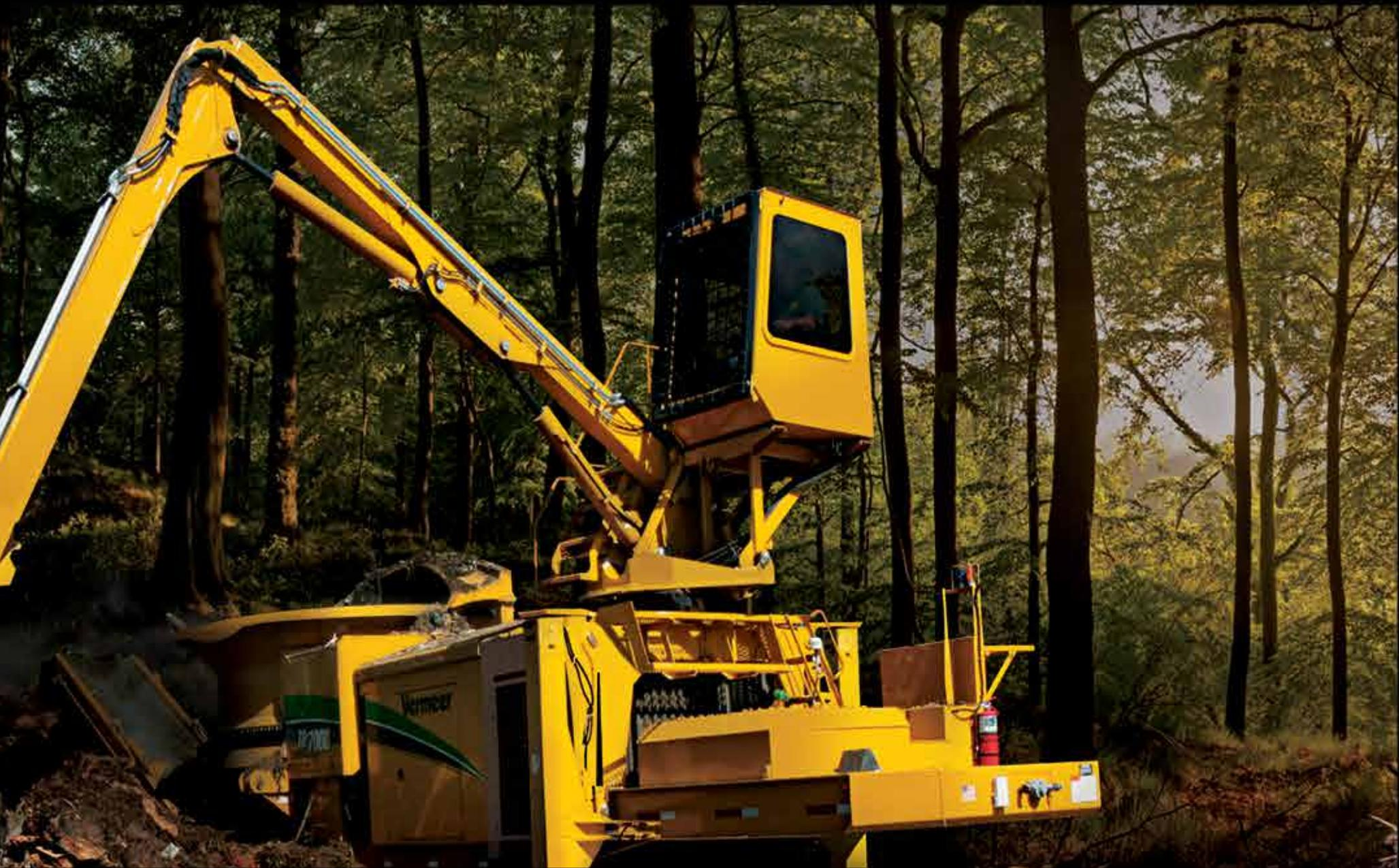
**2: Transportation Package.** A gross weight of 72,300 lb (32,794.7 kg), or 83,300 lb (37,784.2 kg) with loader, the TG7000 has an 11.9' (3.6 m), 20,000 lb (9071.8 kg) triple-axle spread for maximum allowed weight and transportation in the 48 continental U.S.
