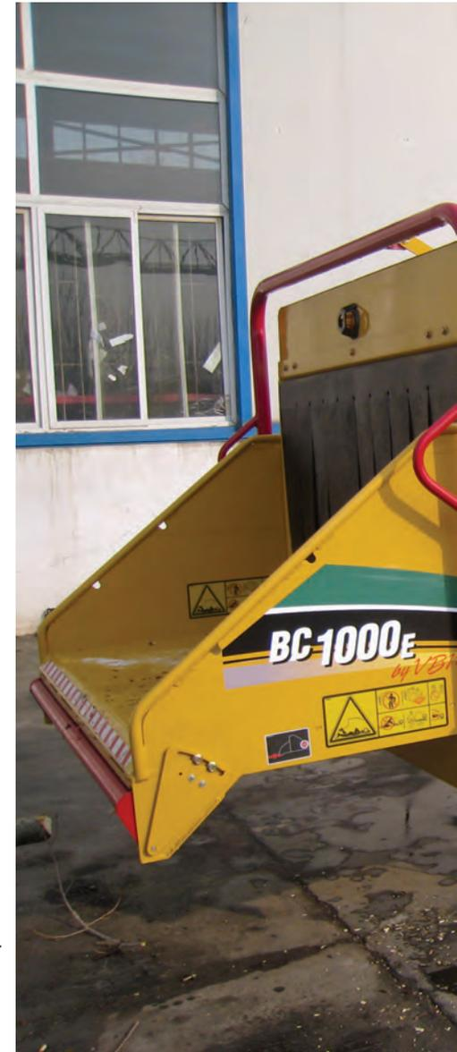
**A large rectangular 30.5 cm x 43.2 cm (12" x 17") feed opening** helps boost productivity by reducing the need to trim material before feeding it into the chipper.
