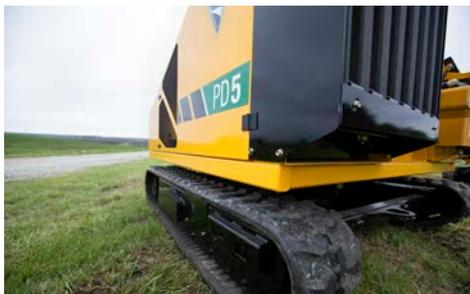
**MOVE ALONG.** With a forward ground drive speed of 2.6 mph (4.18 km/h), the PD5 moves quickly from pile to pile with less time wasted traveling and more time installing piles - keeping your installation efficiently moving forward.
