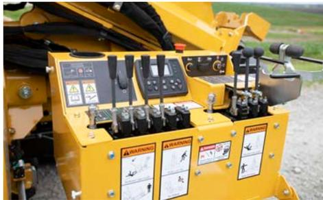
**ON-MACHINE CONTROL.** Walk-beside, machine-integrated controls allow the operator to control machine functions, including engagement of hammer, pile placement and ground drive. Operators remain off the machine and walk beside it, with conveniently placed controls to allow for intuitive operation and operator comfort.
