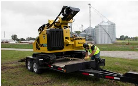
**TRANSPORTATION EASE.** Teardown and transporting is convenient with a rotating platform and a mast that can stay fully assembled and stow parallel with the tracks, making it more convenient for the entire crew to move to the next job.
