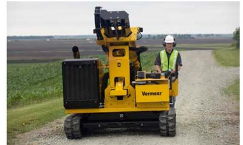
**KEEP IT LIGHT.** The PD5 weighs in at 10,350 lb (4694.7 kg), which allows for transporting up to two pile drivers on select trailers, and less potential damage to jobsites, all while helping increase efficiency of setup and teardown with a lightweight design.
