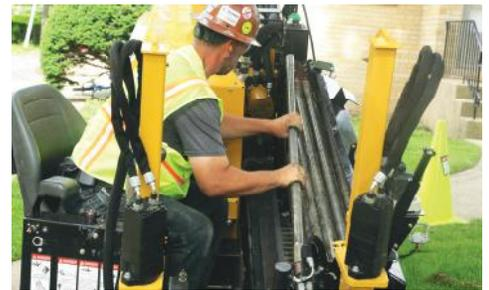
**MULTIPLE ROD OPTIONS.** Equip your drill with either a 6' (1.8 m), 1.66" or 1.31" (4.2 cm or 3.3 cm) Firestick® drill rod and save time on the job with 180' (54.9 m) of on-machine rod carrying capacity.
