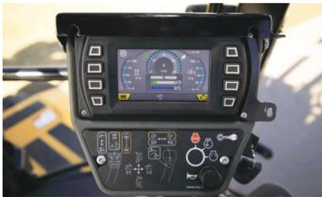
**IMPROVED PRODUCTIVITY.** The RTX1250i2 offers a productivity advantage with classic and newly-added technology like TrenchSense™ electronic control system, Ecolde™ engine control system, Productivity Zone and Auto Plunge.
