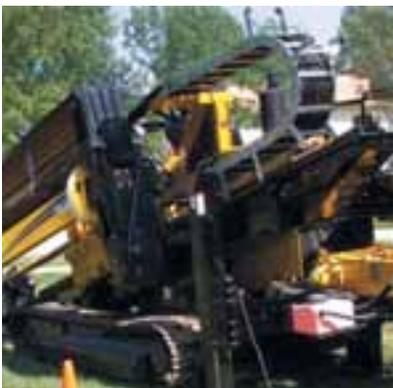
*Rack-and-pinion drive. This system provides for smooth operation. The rack is sectionalized and bolts on for easy repair or replacement.*
