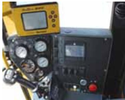
*State-of-the-art operator's station. Dual joysticks control functions for drilling fluid flow, breakout vise and throttle, and are integrated into the thrust and rotation controls. This feature provides the operator fingertip control over repetitive drill functions.*
