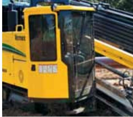
*Climate-controlled cab. The standard cab provides 360-degree visibility for easy monitoring of all machine operations. Independent heating and air-conditioning controls allow the operator to control the cab climate and enhance comfort in all weather conditions, including snow, rain and summer heat. A full-size hinged door provides easy access to the operator's station, while tinted glass windows help reduce glare and heat from the sun.*
