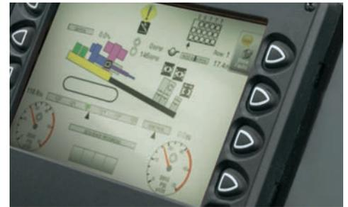
**MAKEUP OR BREAKOUT.** Controls provide options including automated sequence, partially automated sequence or manual sequence of the rod makeup/breakout process, depending upon operator preference and level of expertise.
