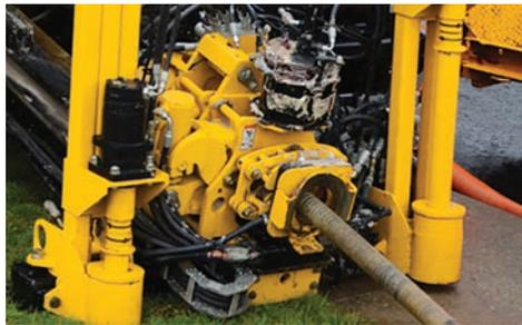
**STAY PRODUCTIVE.** Featuring an exclusive, patent-pending vise assembly consisting of three sets of vises coupled with a control system to optimize productivity and longevity of the drill rod.
