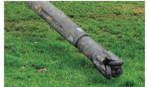
**DRILL BIT OF CHOICE.** Optimize operation in a variety of conditions by choosing from a wide range of drill bits and a specially designed dual rod drill head offered in three different bent sub arrangements.
