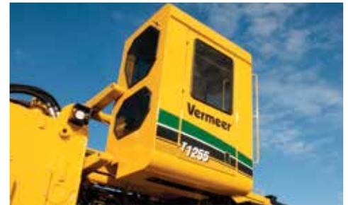
**ELEVATING ENCLOSED CAB.** The elevating cab allows superior visibility and added comfort with the air ride seat. The sealed cab has self-contained heating and air conditioning with sound attenuating foam. It is also a rollover module (ROM).
