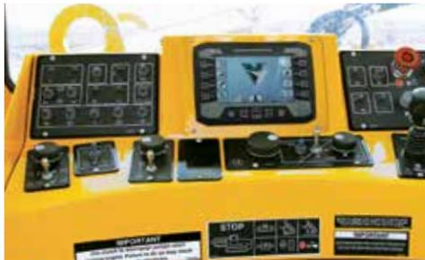
**SMARTTEC ELECTRONIC CONTROL SYSTEM.** SmartTEC performance software helps optimize productivity with real-time machine control prompts. Monitor and record functions encourage proactive machine maintenance and operator performance analysis. Available on all Vermeer TEC® Plus-equipped machines.
