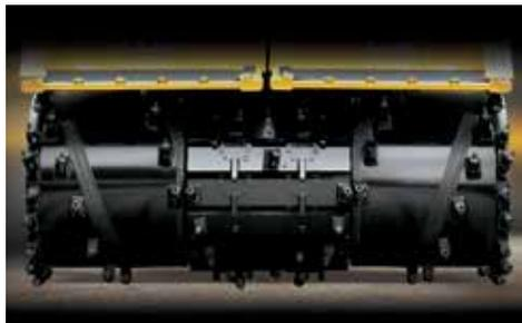
**CHAIN DRIVE TERRAIN LEVELER SEM ATTACHMENT OPTION.** The chain drive Terrain Leveler option gives you the capability to cut along a vertical high wall, with a maximum cutting depth of 27" (68.6 cm).
