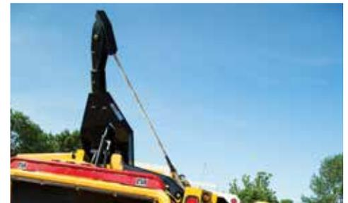
**OPTIONAL WINCH.** Eliminates the need to drag large material to the chipper. The 150' (45.7 m) winch line can handle material up to 4000 lb (1814.9 kg), making it easy to lift logs directly onto the feed table. In addition the winch can also be hydraulically raised out of the way to allow operators to feed the unit using a loader.
