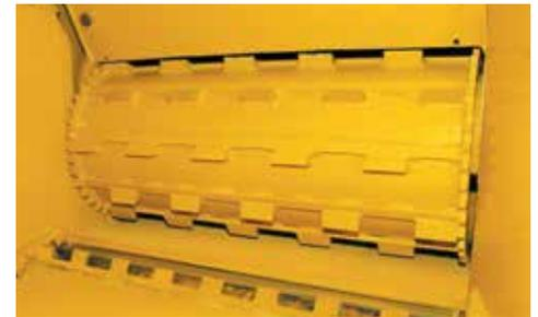
**LOWER FEED ROLLER.** The lower feed roller is offset from the upper feed roller by 10.8" (27.4 cm). Material is easily pulled to the upper feed roller, so there is less need to manually raise the upper feed roller for larger diameter material.
