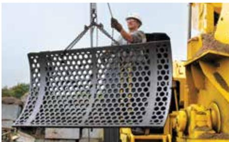
**SIMPLE SCREEN CHANGES.** Operators can change product sizes easily with the onboard screen handler system.
