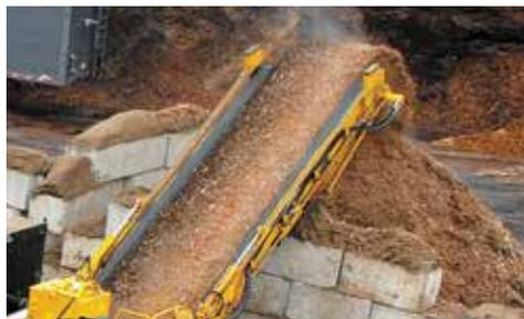
**HIGH PRODUCTION.** Yield higher volumes of wood waste and reduce spillage or plugging due to a 66" (167.6 cm) wide loadout conveyor, with a discharge height of 14' to 18' (4.3 m to 5.5 m).
