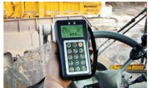
**REMOTE CONTROL.** Discharge height, along with several other machine functions, is adjustable via remote control.
