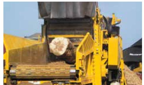
**INCREASE INPUT.** Process larger or irregularly shaped wood waste due to a class-leading 50" x 71.5" (127 cm x 181.6 cm) infeed opening. Four preset infeed settings help control the material's finished size.
