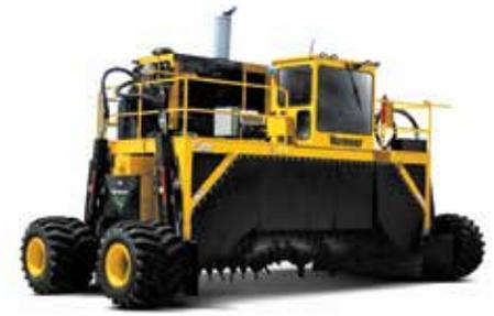
**EASE OF MAINTENANCE.** All grease points are accessible from ground level. Hinged, lockable doors on both sides of the engine provide spacious access for maintenance.
