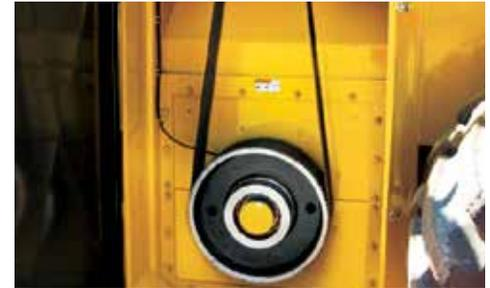
**RELIABLE COMPONENTS.** The poly-synchronous belt drum drive has proven to be a reliable system requiring little maintenance and offering adjustable shafts.
