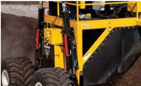
**PRECISE CONTROL.** Equipped with independently controlled lift cylinders for thorough aeration of the compost pile.
