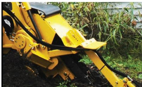
**MAKE SENSE OF YOUR TRENCH.** When difficult conditions are encountered while trenching, causing a sudden drop in engine speed, the TrenchSense™ electronic control system automatically pauses the forward motion of the tractor to prevent engine shutdown and recalibration of the machine controls. Once preset engine and trencher speed recovers, forward AutoCreeep resumes. The sequence occurs within seconds and requires no operator adjustment.
