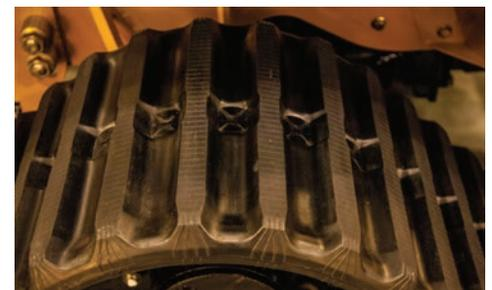
**QUAD TRACK SYSTEM.** The quad track system offers improved flotation, reduced surface damage and increased tractive effort. Four-wheel steer and crab steering are functional with both quad track and tire options.
