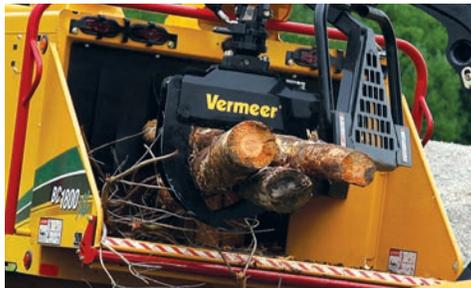
**CHIPPING PRODUCTIVITY.** The SmartFeed system monitors engine rpm and automatically stops and reverses the feed rollers to enhance production. This system also senses feed roller jams and manipulates the material automatically to reduce the need for manual control bar use.
