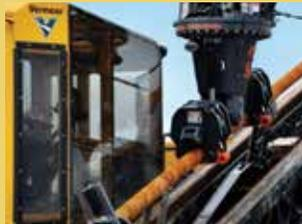
*Features load hold valves on grab arm cylinders to keep arms locked and loads secure in case of hydraulic failure.*
