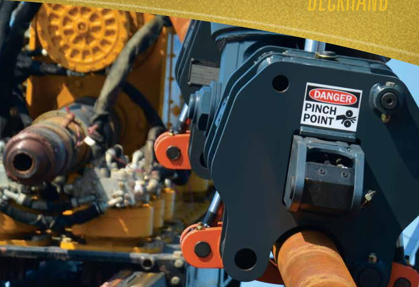
Get it done in all conditions. The *DECKHAND*® HDD arms handle drill pipe in a range of surface conditions. *DECKHAND*® HDD arms can carry 3.5" (8.9 cm) to 9.5" (24.1 cm) diameter drill pipe, loading pipe on or off trailers, pipe racks or drill rigs.
