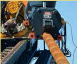
*Handles pipe from a center and off-center position, reducing transfer time for each load.*
