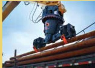
*Achieves +/- 19 degree tilt along the main beam to more easily match angled pickup or drop-off points.*
