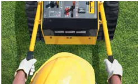
**VZ STEERING.** Instead of additional levers and steerable wheels, operators can turn the machine using only the handlebars. These bars also provide additional leverage when operating in difficult terrain.
