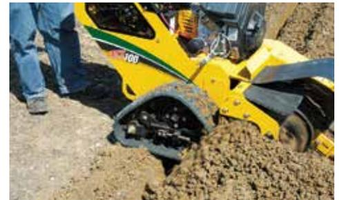
**HYDRAULIC SYSTEM.** The RTX100 is equipped with a tandem hydrostatic ground drive pump with a separate attachment pump which produces a dedicated 8 GPM (30.28 LPM) to the trencher circuit.
