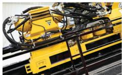
POWERFUL TORQUE. Operators can adjust the drill from 30,000 ft-lb to 52,600 ft-lb (40,675 Nm to 71,316.1 Nm) of rotary torque, with maximum torque being highly advantageous when turning large-diameter reamers and hole openers for installing large-diameter product.
