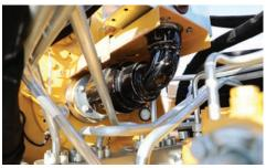
MUD FLOW. The enhanced water course system features four 1.5-in (3.8-cm) mudlines and a 3-in (7.6-cm) head shaft, allowing high volumes of fluid to be pumped downhole.
