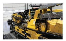
**CARRIAGE SPEED.** The high carriage speed aids in fast rod cycle time when adding or removing drill rods and helps cut down on cycle time when tripping out of the borehole.
