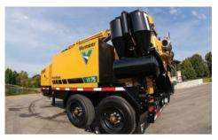
CYCLONIC FILTRATION. The dual cyclonic filtration uses a tuned vortex system in which the outer vortex spiral forces small particles to fall into a separate canister.
