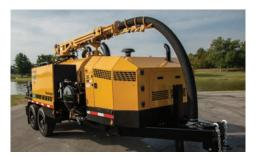
HYDRAULIC BOOM (OPTION). 5 in (13 cm) diameter with a 14 ft (4.3 m) reach. Exclusive telescoping boom maintains hose length during extension and incorporates a remote controlled hydraulic valve for vacuum shut off.
