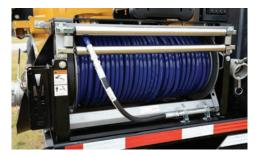
SEWER JETTER (OPTION). The sewer jetter system turns your Vermeer vacuum system into a versatile jetter/vac combination unit. It is available with 18 gpm (68 L/min) at 2,000 psi (138 bar) with 500-ft (152-m) x .5-in (13-mm) jetter hose.
